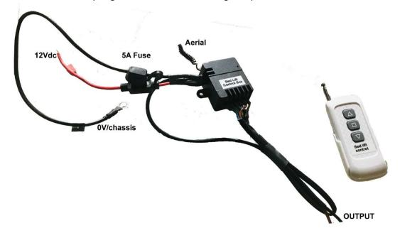
The output cables are sleeved in red and black. They correspond to the red and black of the actuators flying leads. The actuators flying leads will need to be extended to your exact needs.
